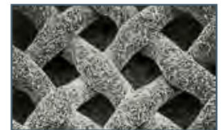
After sandblasting, bracket base is more porous, increasing bond strength
